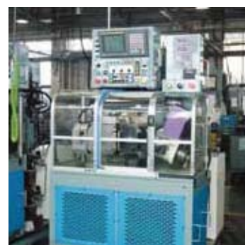
傘歯切盤小型NC Formate 自社開発 Nissei NC Formate Bevel Gear Cutting Machine
