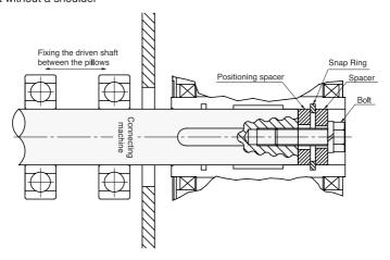
Figure-4 Fixing by spacer and snap ring
