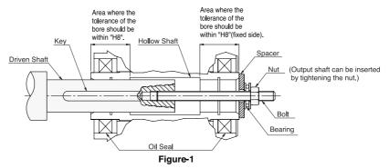
(Spacer, nut, bolt, key and other parts for bearing should be prepared by customer.)
