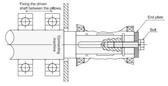
Figure-3 Fixing by End plate
