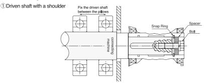
Figure-2 Fixing by spacer and snap ring
