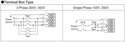
MS: Electro-Magnetic Switch C: Capacitor
