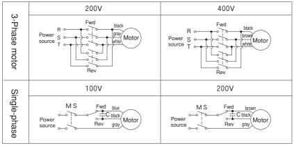
MS: Electro-Magnetic Switch C: Capacitor
