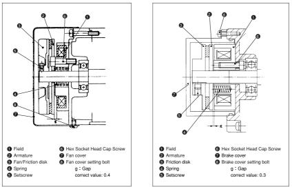
After operation for an extended period of time, the brake gap(g) become greater than 0.8mm, making it impossible to release the brake.
