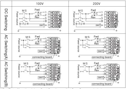
MS : Electro-Magnetic switch C : Capacitor -N-: Surge Suppressor (option)
